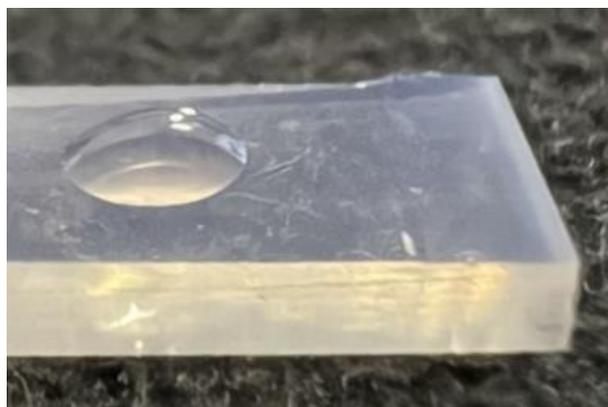
Fig. 1. A photograph of the surface of a laser-densified PS sample taken a few minutes after the application of a drop of water.
